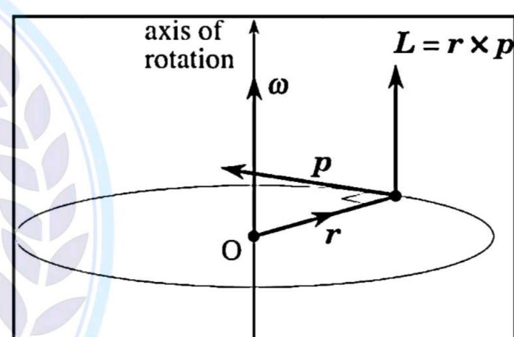
The direction of angular momentum is normal to the plane formed by  $\vec{r}$  and  $\vec{P}$  as given by right hand rule.
