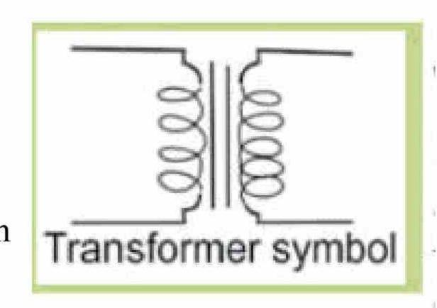
Types of Transformer: There are following types of transformer Step-up transformer: Such a trtransformer in which voltage across thethe secondary is greater than primary voltage is cacalled step up transformer as Ns>Np p so Vs>Vp. Step-down transformer: Such uch a transformer in which voltage acrossoss the secondary is less then primary voltage is callecalled step down transformer. Ns<Np, Vp, Vs<Vp.
