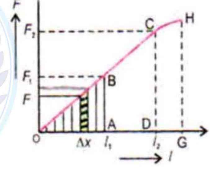
$$E = \frac{Stress}{Strain} = \frac{F_1}{I_1} = \frac{F_1L}{AI_1}$$
