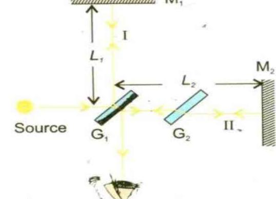
**Explanation**: let us consider a monochromatic light from a light source falls on half silver glass plate G1(beam splitter) G1 that partially reflects it and partially transmit it towards the fixed and moveable mirror. Both beams reflects from both mirrors and interfere constructively and destructively observed by observer's eye through telescope. If mirror is moved
