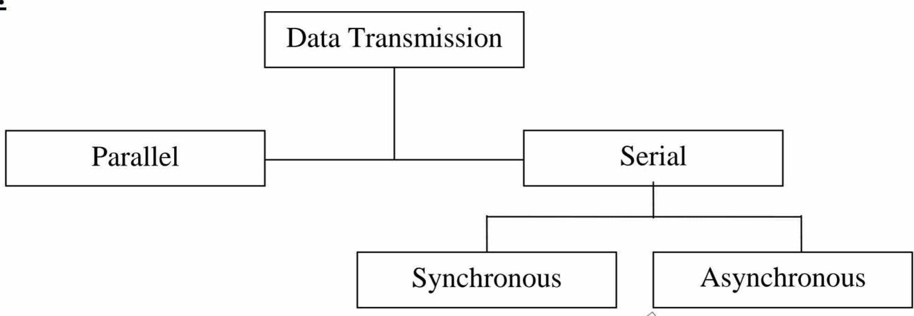
**Parallel Data Transmission**: [Concurrent flow of bits of data through separate communications lines.] This pattern resembles the flow of automobile traffic on a multilane highway. Parallel data transmission is commonly used for interactions between a computer and its printer.
