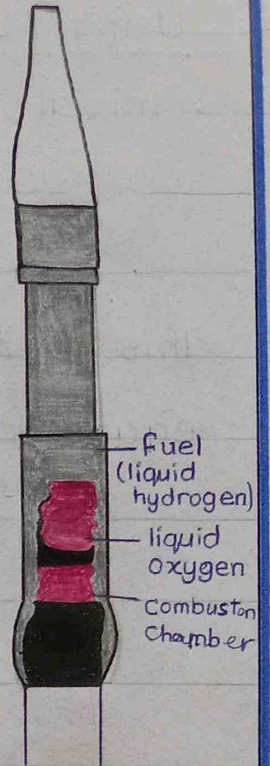
A rocket carries its own fuel in the form of a liquid or solid Hydrogen and Oxygen.
