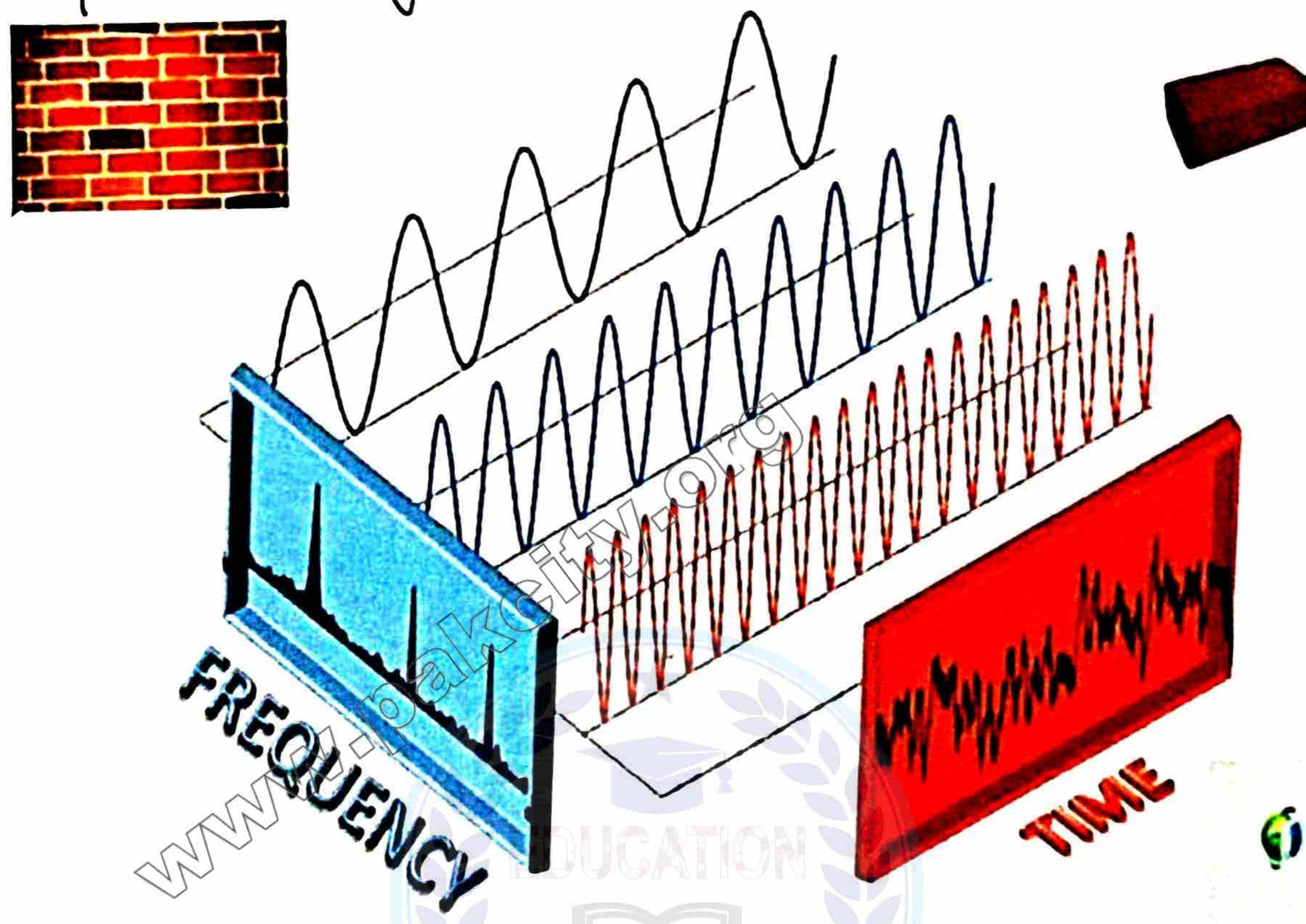
The above Process is called Fourier Transformation And it is helpfull in Mobile Application, Radar and Channel Modeling.
