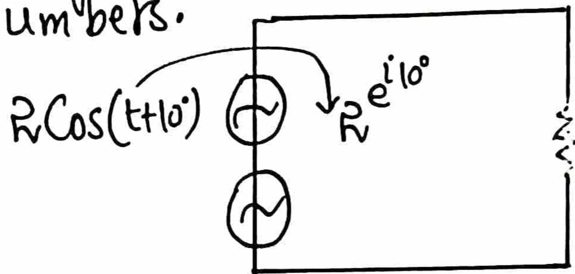
When we put Capacitor and inductor into a Circuit, that will shift Voltage and Current depending upon the values. Math represents that it is all due to Complex Numbers. We Use Imaginary Numbers to determine the shift in the Circuit.
