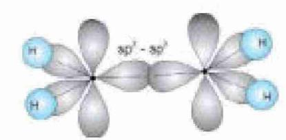
Overlap of orbitals:  $sp^2$  hybrid orbital of each carbon overlaps to give  $sp^2-sp^2$  sigma bond and the other two  $sp^2$  orbitals overlap with 1s orbitals of hydrogen to give  $sp^2-s$  sigma bonds. The unhybridized 2pz orbitals overlap sideways to give a  $\pi$ -bond.
