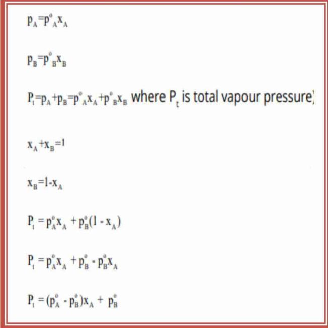
Two liquids 'A' and 'B' with vapour pressures  $p_A^a$  and  $p_B^a$  in the pure state at a given temperature.
