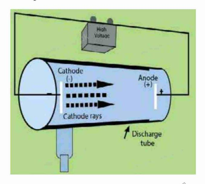
Cathode and anode connected to negative and positive terminals of the battery, respectively.
