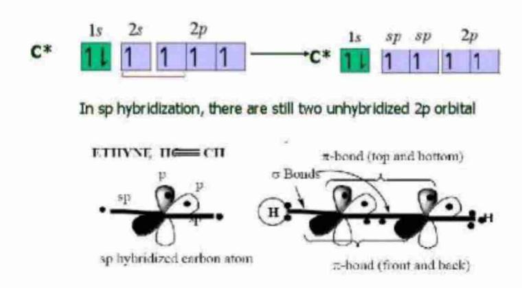
Overlap of orbitals: Two sp hybridized carbon atoms join together to form a sigma bond by sp-sp overlap. The other sp orbital forms a sigma bond with 1s orbital of hydrogen atom. The two unhybridized p orbitals on each carbon atom overlap sideways give two  $\pi$  -bonds.
