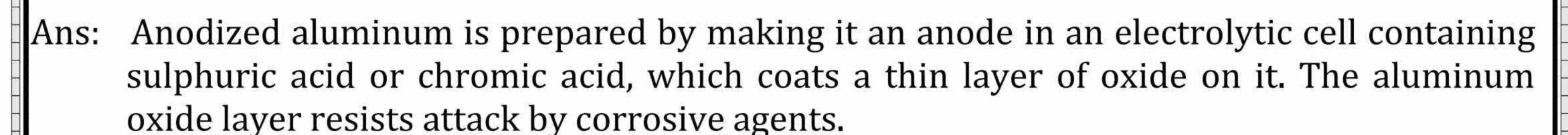
The freshly anodized aluminum is hydrated and can absorb dyes.
