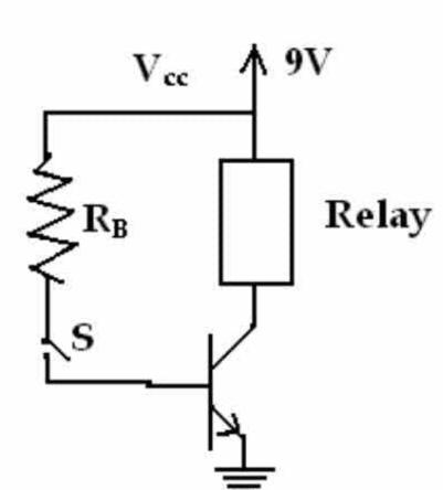
18.3: In circuit (Fig.P.18.3), there is negligible potential drop between B and E, where  $\beta$  is 100, calculate (i) base current (ii) collector current (iii) potential drop across  $R_c$  (iv)  $V_{CE}$ .
