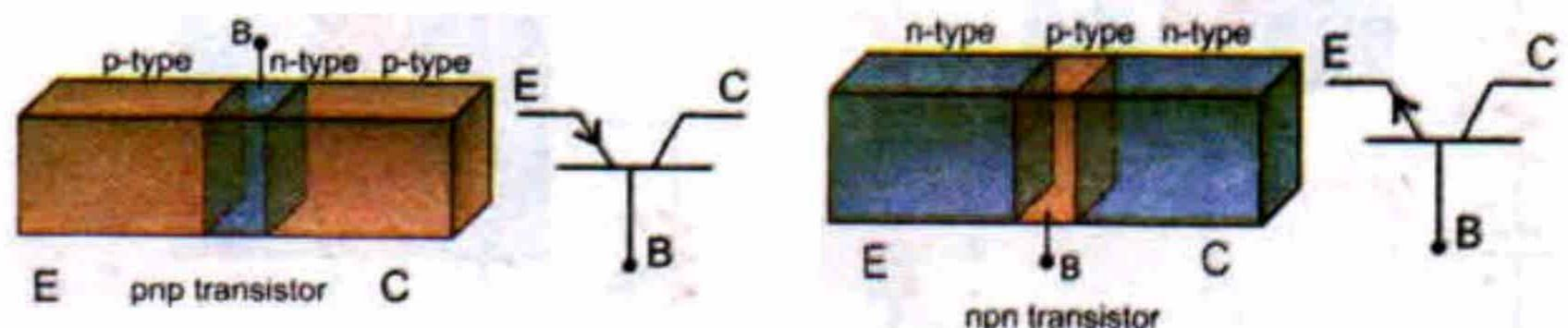
**p-n-p transistor**: Such type of transistor in which n type substance is sandwiched b/w two p type substances is called p-n-p transistor.
