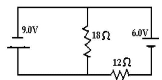
Let I<sub>1</sub> & I<sub>2</sub> are the current flowing through loop in CW direction
