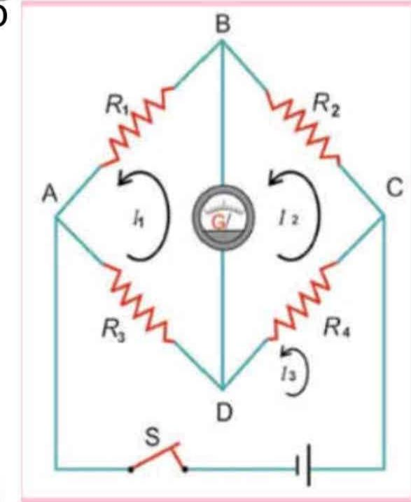
$$\frac{-I_1R_1}{-I_2R_2} = \frac{I_1R_3}{I_2R_4} \implies$$
