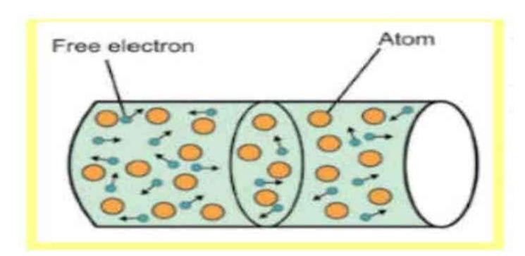
Current through metals when battery is connected:
