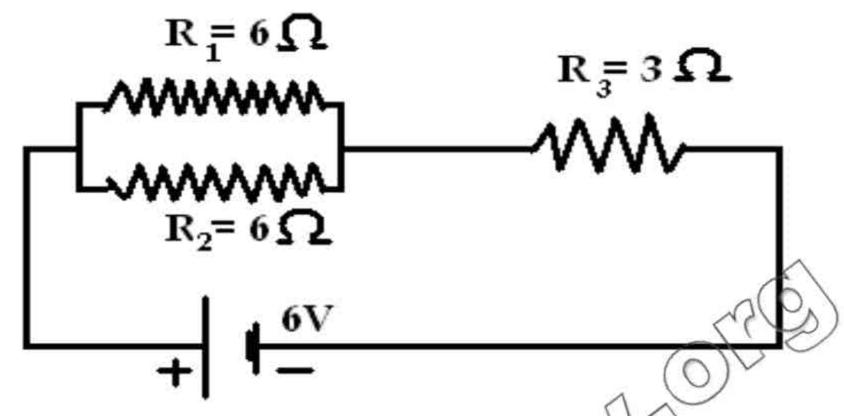
Data:  $R_1 = 6\Omega\Omega R_2 = 6\Omega\Omega R_3 = 3\Omega\Omega V = 6V$ , Re' = ?, I = ?,  $I_2 = ?$
