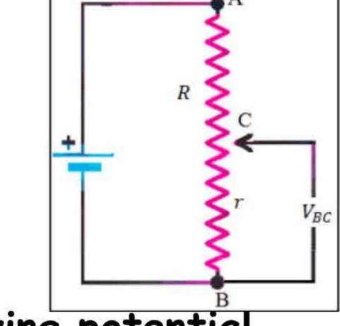
7. \*\*Describe a circuit which will give a continuously varying potential.
