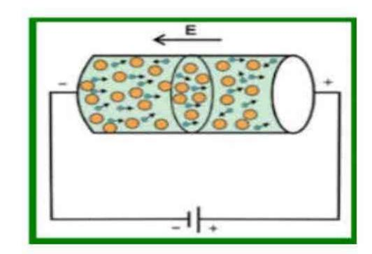
**<u>Drift Velocity</u>**: "Average constant velocity of free electrons inside the metallic conductors in opposite to electric field intensity is called drift velocity". Its value is 10<sup>-3</sup> m/s.
