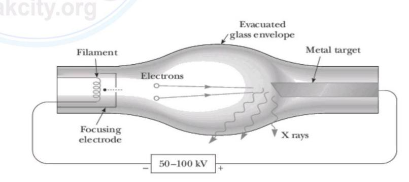
high atomic number). If potential difference is of several thousand of volt X-rays are emitted out of the anode.
