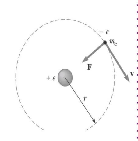
As the electron is revolving in a circular orbit of radius the exists a centripetal force acting on it given by;
