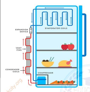
**<u>Principle</u>**:- Its basic principle is evaporation and compression.
