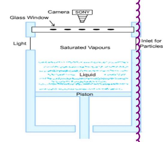
A movable piston on the bottom. The piston can be moved up or down by a lever attached to it.
