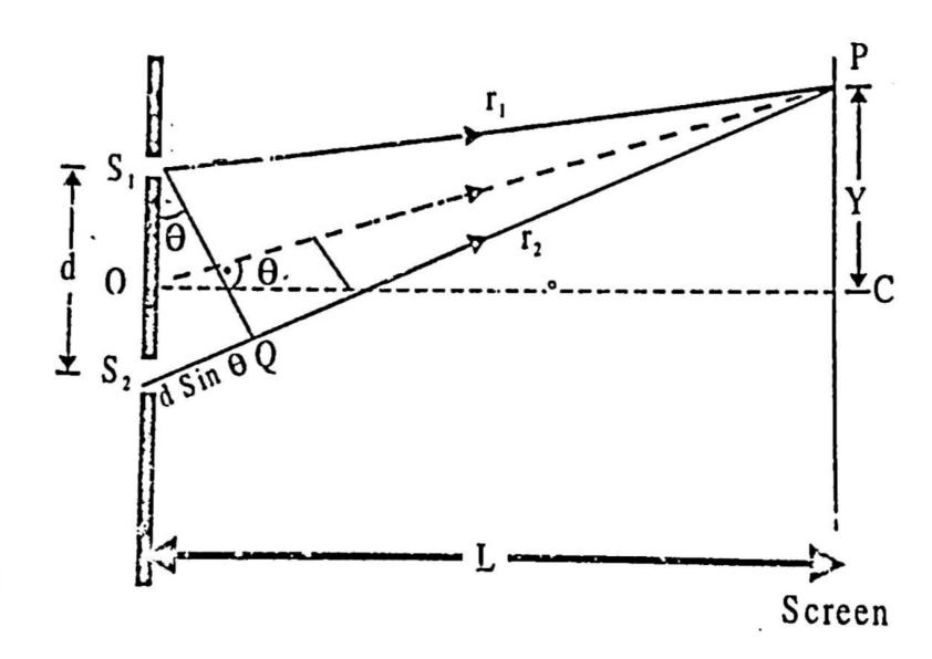
If O be the central point on the screen then the path difference between  $S_1O$  and  $S_2O$  will be zero and the constructive interference will take place at O.
