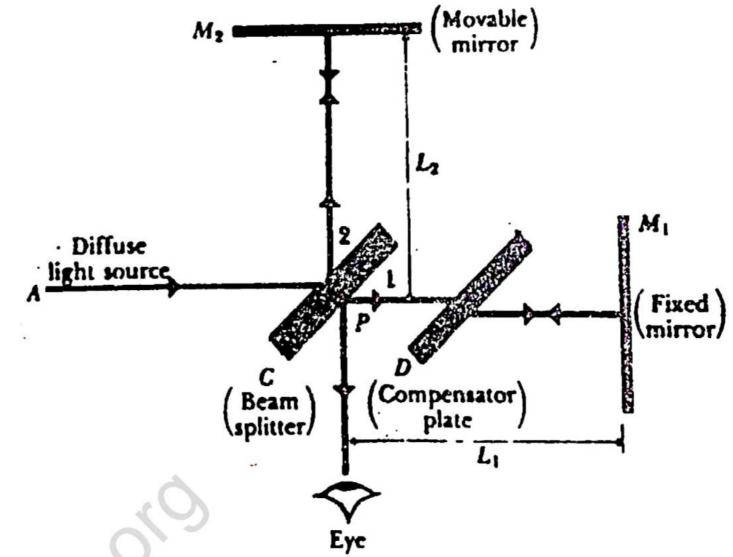
from the mirror M<sub>2</sub>. It then returns through D and I reflected from the silvered surface of C to the observer eye. Both the plates C and D are of early same thickness so that the rays 1 and 2 through the same thickness of glass. The plate C is called beam splitters.
