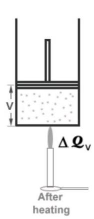
Above equation represent Isochoric process. So, in isochoric process heat supplied to the system is used completely to change the internal energy.
