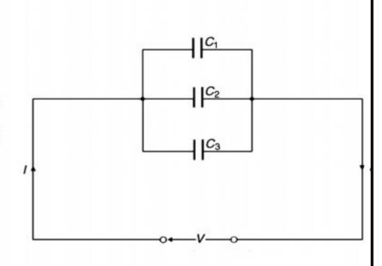
Consider three capacitors  $C_1$ ,  $C_2$ ,  $C_3$  connected in parallel. A charge q given to a point divide itself resides on the plates of individual capacitor as  $q_1$ ,  $q_2$ ,  $q_3$  respectively.
