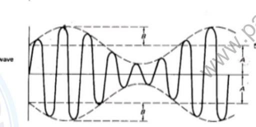
$$M = \frac{Amplitude \ of \ modulating \ signal \ (volts)}{Amplitude \ of \ carrier \ signal \ (volts)} \times 100$$
