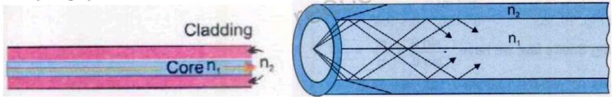
Single-mode fiber is preferred in telecommunications because they are digital and use monochromatic laser light. Here the transmission is free from dispersion.
