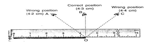
PARALLAX ERROR:- The error which occurs due to incorrect position of the eye is known as parallax error as shown in figure.
