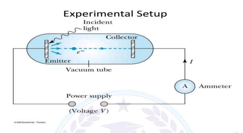
Suppose that we now reverse the potential difference between the electrodes so that the target material now connects with the positive terminal of a battery, and then we slowly increase the voltage. The photocurrent gradually dies out and eventually stops flowing completely at some value of this reversed voltage. The potential difference at which the photocurrent stops flowing is called the **stopping potential**.
