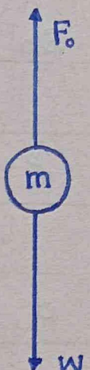
At any instant when the drag force becomes equal to its weight. Then the droplet moves with constant velocity which is known as terminal velocity.
