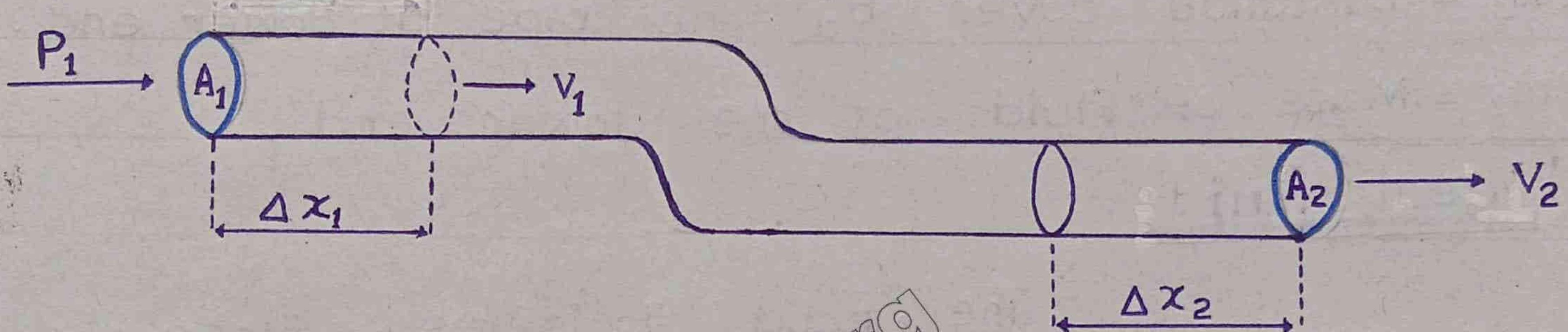
Consider a fluid moving through the horizontal pipe along stream line flow.
