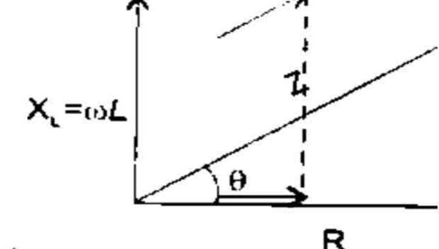
7. A choke coil placed in series with an electric lamp in an A.C. circuit causes the lamp to become dim. Why is it so? A variable capacitor added in series in this circuit may be adjusted until the tamp glows with normal brilliance. Explain, how this is possible?
